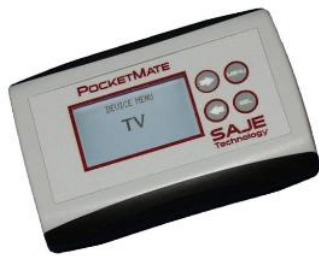
Switch Scanning Environmental Control Unit
